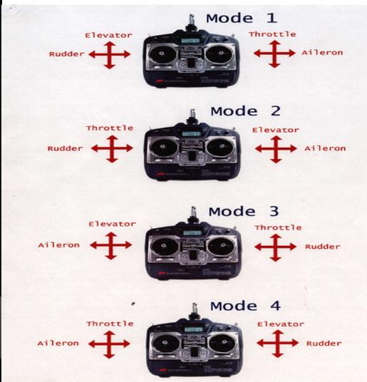
Press Phone or Tablet " Menu" ---> " Set", the Tx mode can be available to setup, and you can select the Tx mode according to your operation preference. Then the Tx stick display on GCS will change following Tx mode changing.
