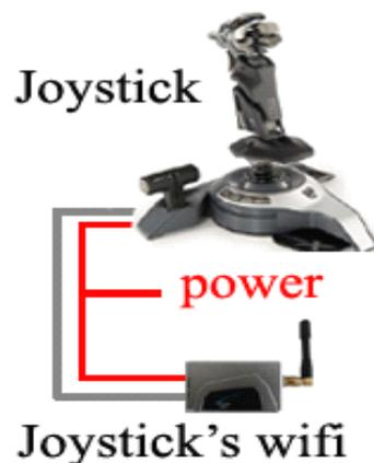
The joystick connection is quite simple, just connect joystick WIFI to joystick according to the figure above, then power it on in a convenient place , joystick can work automatically .
