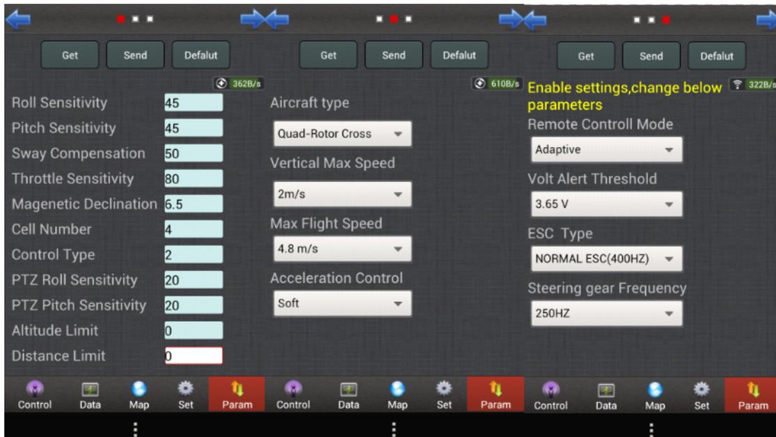
Notice: "Roll Sensitivity" & "Pitch Sensitivity" (default 45) may directly affect the manual reaction. "Motion compensation" (default 80) can improve stabilization but reduce the reaction. Throttle sensitivity (default 80) may affect Altitude control sensitivity, choose the max. speed of copter climb or decline among 2m/s, 4m/s and 5m/s in "Max. Vertical Speed" bar.
