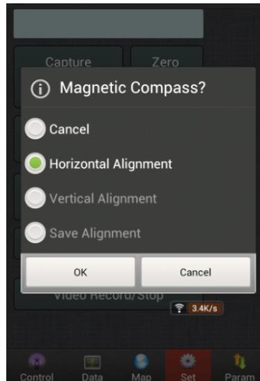
Point the front of the Multi down and get the blue LED light on. Now turn slowly clockwise 2-3 times in one spot ensuring the light remains on at all times and the moving data of Attitude Angle remains within 3 deg.
