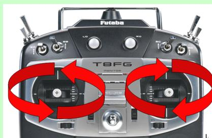
Then observe the diagram of Manual Servo Position on GCS user interface to check whether it is the same as the real Tx operation, if same the Tx operation is correct, if not same please set Tx channel to be inverted.
