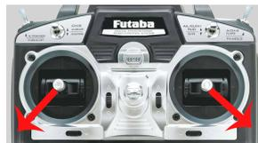
**With motor started, the copter does not fly by pushing throttle stick a little and certain motor may move slowly and even stop, it is normal phenomenon caused by multi-rotor integral for adjusting attitude. Throttle up then can keep flying started immediately.**
