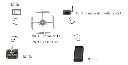
In PTP mode, Mobile and WIFI communicates directly and no need to prepare extra router.
