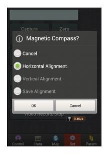
Point the front of the Multi down and get the blue LED light on. Now turn slowly clockwise 2-3 times in one spot ensuring the light remains on at all times and the moving data of Attitude Angle remains within 3 deg.
