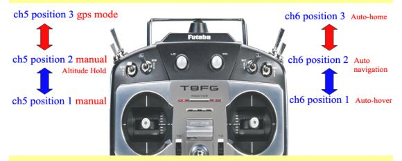
The RC receiver on aircraft may be switched on/off by the button "Receiver on" and "Receiver off" in Setting section(GCS). Tx operations do not work on aircraft with RC receiver switched off (when the two buttons Receiver on/off shall get green ), i.e. There is no receiver installed on craft.
